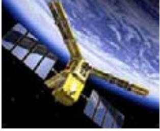
The SMOS satellite with radiometer 'blades' for measuring Soil Moisture and Ocean Salinity (SMOS). This mission has been designed to observe soil moisture over the Earth's landmasses and salinity over the oceans. Soil moisture data are urgently required for hydrological studies and data on ocean salinity are vital for improving our understanding of ocean circulation patterns.
